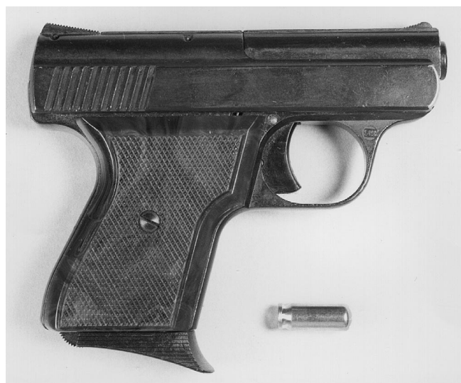
Fig. 1 The starter's pistol used in case 1: Rhöner, mod. SM 15, cal. 8 mm, PTB-No. 83. Underneath the muzzle an 8 mm blank cartridge
